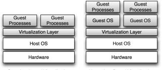
Container-based Virtualization Hypervisor-Based Virtualization
