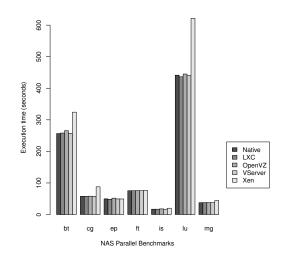
Figure 5. Single node comparison of NPB performance overhead.
