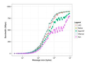
Figure 3. Network bandwidth using NetPIPE.
