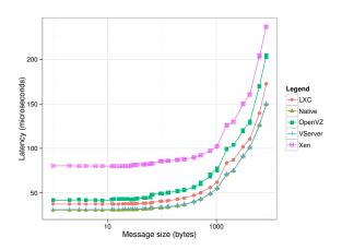
Figure 4. Network latency using NetPIPE.
