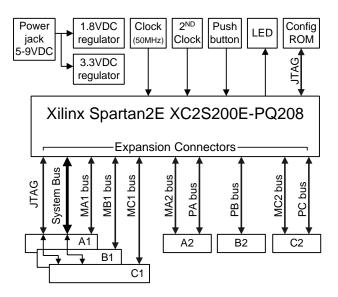
Figure 1. D2-SB Circuit Board Block Diagram
