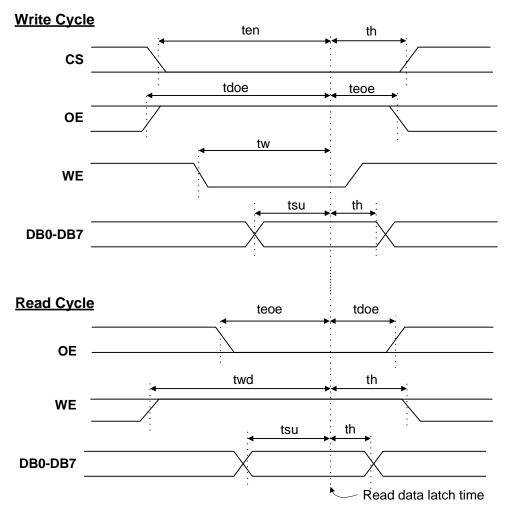
Figure 3. System Bus Timing
