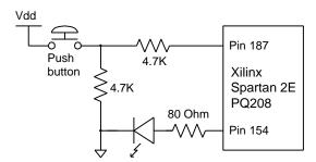
Figure 2. Pushbutton and LED Circuit
