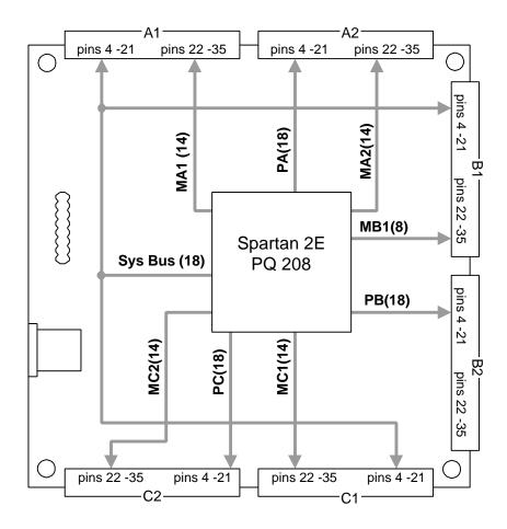
Figure 4. Expansion Connector Signal Routing
