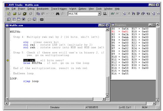
Using key F5 of the studio we multistepped over these loops to a breakpoint at the end of the multiplication routine. The result register pair R4:R3 has the result of the multiplication of 0xAA by 0x55: 0x3872.
