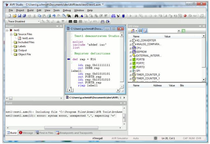
On the left, the project window allows you to manipulate and view all your project files. In the middle, the editor window, allows you to write your source code (try typing its content to your editor window, don't care about the colors – these are added by the editor – remember syntax-highlighting?). On the left bottom is a "Build" section, where all your error messages go to. On the right side is a strange I/O view and below a rather white field, we'll come to that later on.
