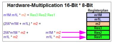
So the 16-bit-binary m1 is equal to 256\*m1M plus m1L, where m1M is the MSB and m1L is the LSB. Multiplying m1 by 8-bit-binary m2 so is, mathematically formulated:
