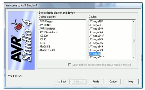
As debug platform select either "AVR simulator" "AVR or simulator 2". As Device select your AVR type, here an ATmega8 selected. If your desired type is grayed out, select another simulator platform. Close this window "Finish" with the button. Now a large window pops up, which has lots of different windows
