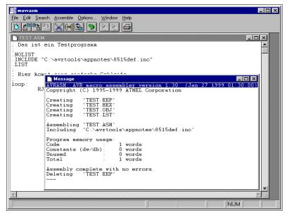
Clicking on the editor's external program caller or on the batch file starts the command line assembler. That piece of software reports the complete translation process (in the smaller window), here with no errors. If errors occur these are notified, along with their type and line number. Assembling resulted in one word of code which resulted from the RJMP instruction that we used. Assembling our single asm text file now has produced four other files (not all apply here).
