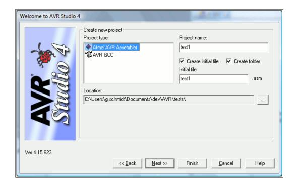
Here you select "Atmel AVR Assembler" as your project type, give that project a name (here "test1") and let the Studio crate an initial (empty) file for your source code, let it create a folder and select a location for that project, where you have write access to.
