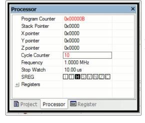
The cycle counter of the multiplication points to 10, at 1 MHz clock a total of 10 microseconds. Very much faster than software multiplication!
