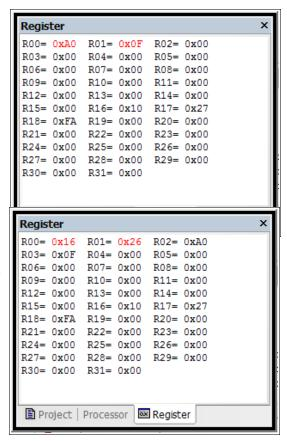
Now two steps are performed at once: multiplication by 256 and adding the result to the previous result. This is done by adding R1:R0 to Res3:Res2 instead of Res2:Res1. R1 can just be copied to Res3. R0 is added to Res2 then. If the carry is set after adding, the next higher byte Res3 is increased by one.
