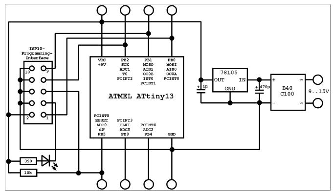
The ATtiny13 requires no external XTAL or clock generator, because it works with its internal 9.6 MHz RC generator and, by default, with a clock divider of 8 (clock frequency 1.2 MHz).
