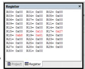
$Multiplying the two \, MSBs \, (hex \, 27 \, and \, 61) \, and \, copying \, the \, result \, in \, R1:R0 \, to \, the \, two \, most \, upper \, result \, registers \, R5:R4 \dots \, (limits a limit of limits and limits a limit of limits a limit of limits and limits a limit of limits a limit of limits and limits a limit of limits a limit of limits and limits a limit of limits a limit of limits and limits a limit of limits a l$
