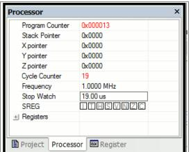
cycles, which is very much faster than with software multiplication. Another advantage here: the required time is ALWAYS exactly 19 cycles, and it doesn't depend on the input numbers (like is the case with software multiplication and on overflow occurrences (thanks to our small trick of adding zero with carry). So you can rely on this ...
