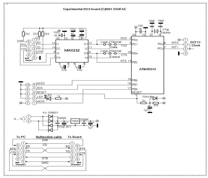
The easiest output device can be a LED, connected via a resistor to the positive supply voltage. With that, you can start writing your first assembler program switching the LED on and off.
