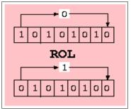
For understanding the multiplication operation, it is necessary to understand the binary rotation instructions ROL and ROR. These instructions shift all bits of a register one position left (ROL) resp. right (ROR). The void position in the register is filled with the content of the carry bit in the status register, the bit that rolls out of the register is shifted to this carry bit. This operation is demonstrated using 0xAA as an example for ROL and 0x55 as an example for ROR.
