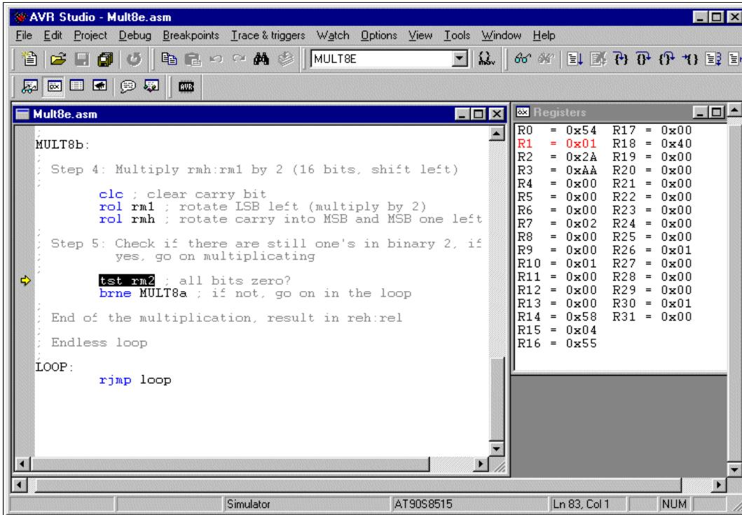
Using key F5 of the studio we multi-stepped over these loops to a breakpoint at the end of the multiplication routine. The result register pair R4:R3 has the result of the multiplication of 0xAA by 0x55: 0x3872.
