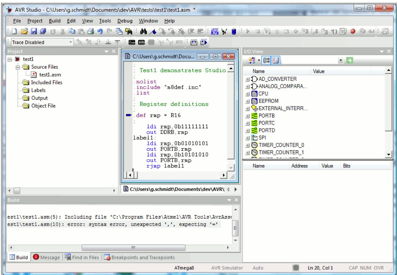
On the left, the project window allows you to manipulate and view all your project files. In the middle, the editor window, allows you to write your source code (try typing its content to your editor window, don't care about the colors – these are added by the editor – remember syntax-highlighting?). On the left bottom is a "Build" section, where all your error messages go to. On the right side is a strange I/O view and below a rather white field, we'll come to that later on.
