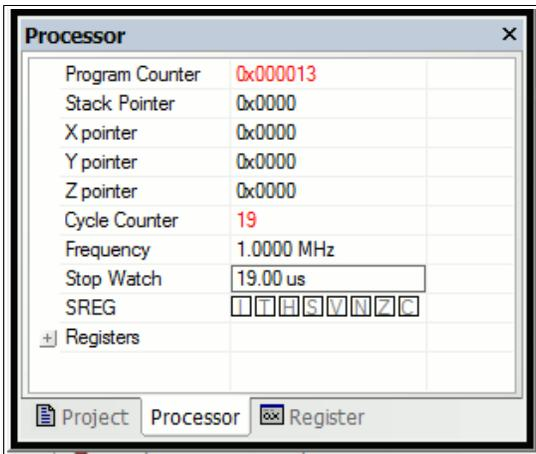
Multiplication needed 19 clock cycles, which is very much faster than with software multiplication. Another advantage here: the required time is ALWAYS exactly 19 cycles, and it doesn't depend on the input numbers (like is the case with software multiplication and on overflow occurrences (thanks to our small trick of adding zero with carry). So you can rely on this ...
