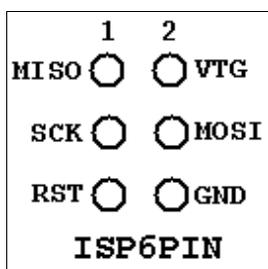
These three signal pins are internally connected to the programming machine only if you change the RESET (sometimes also called RST or restart) pin to zero. Otherwise, during normal operation of the AVR, these pins are programmable I/O lines like all the others.
