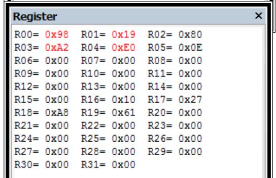
Multiplying the LSB of m1 with the MSB of m2 and adding the result in R1:R0 to the result register's two middle bytes, no carry occurred. The result is hex 0EE6B280, which is 250000000 and obviously correct ...
