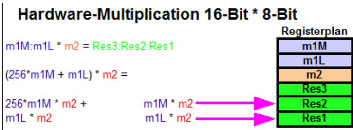
So the 16-bit-binary  $m1$  is equal to  $256 * m1M + m1L$ , where  $m1M$  is the MSB and  $m1L$  is the LSB. Multiplying  $m1$  by 8-bit-binary  $m2$  so is, mathematically formulated:
