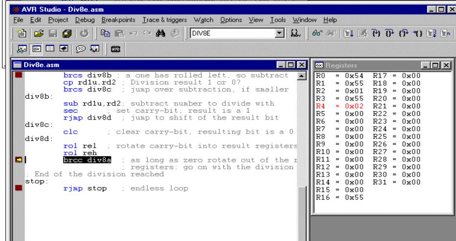
No overflow from rotation into carry has occurred and 0x01 in R2 was smaller than 0x55 in R3, so subtraction was skipped. A zero in the carry is rotated into the result register R5:R4. The former content of the result register, a single 1-bit in position 0 has rotated to position 1 (content now: 0x0002). As a zero was rotated out of the result register pair, the next step to be executed is a branch to the beginning of the division loop start and the loop is repeated.
