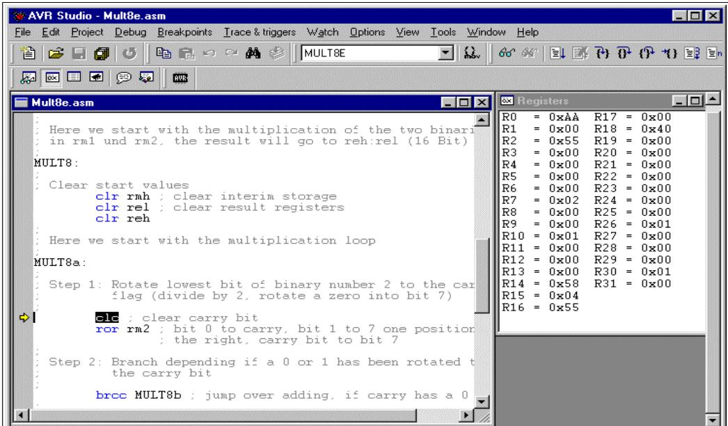
R2 is rotated to the right, to roll the least significant bit into the carry bit. 0x55 (0101.0101) yielded 0x2A (0010.1010).
