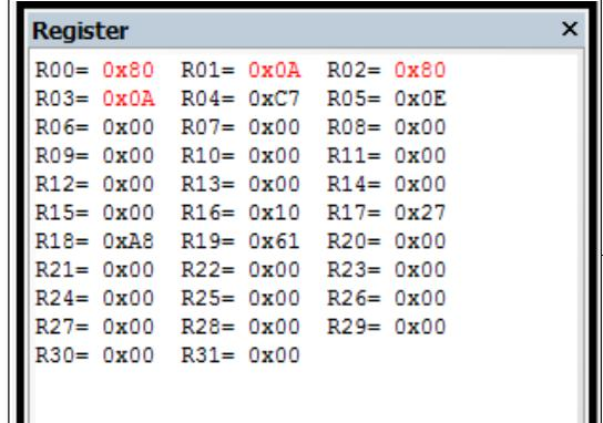
Multiplying the MSB of m1 with the LSB of m2 and adding the result in R1:R0 to the result register's two middle bytes, no carry occurred ...
