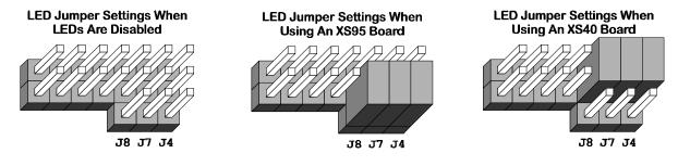
Figure 3: Shunt placement for setting the XStend Board LED supply voltages.
