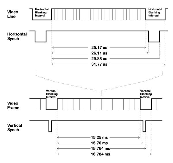
Figure 10: VGA signal timing.
