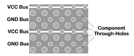
Figure 5: Top-side view of the network of VCC and GND buses around the component through-holes in the XStend Board prototyping area.
