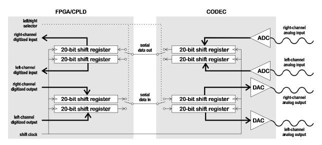
Figure 13: Connections between the XStend codec chip and the XS Board FPGA or CPLD.
