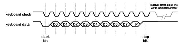
Figure 12: Keyboard data transmission waveforms.
