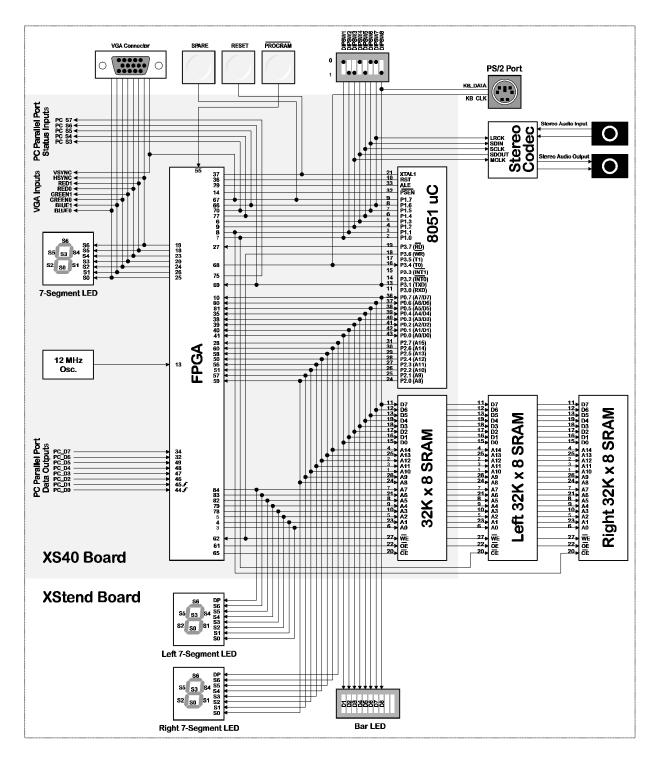
Figure 7: Programmer's model of the XS40/XStend Board combination.
