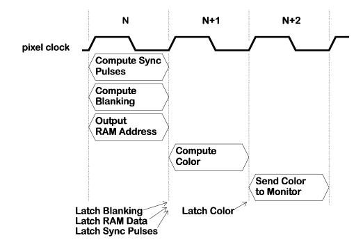
Figure 11: Pipelining of VGA signal generation tasks.
