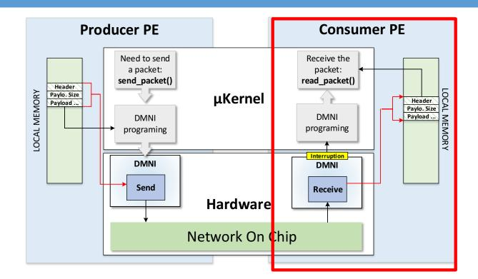
read\_packet(): function that programs the DMNI to copy a NoC packet to a memory block
