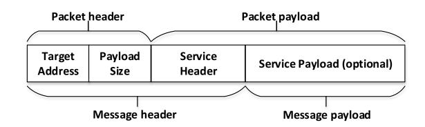
From the NoC point of view, the packet has a **header** and a **payload**
