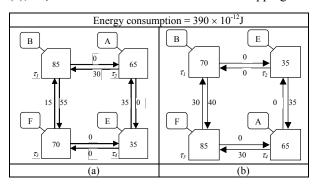
Figure 2 – Mappings for Figure 1(c, d) - estimation of energy consumption obtained with CWM.
