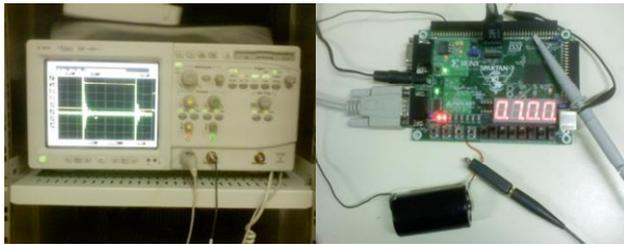
**Fig. 7 DPA/CPA Measurement setup.**
