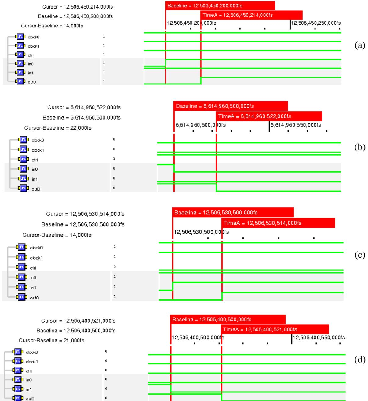
**Figure 4.36 – Timing simulation results for a gate level design of a single 2 input C-Element standard cell. (a) and (b) presents, respectively, rise and fall propagation delays from pin *A* to *Q*, while (c) and (d) presents the propagation delays from pin *B* to *Q*.**
