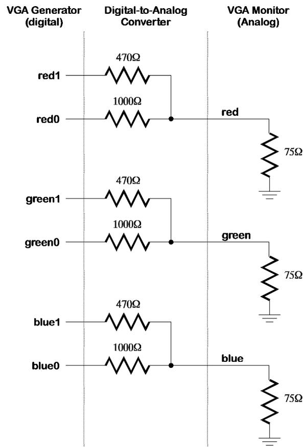
**Figure 9:** Digital-to-analog interface to a VGA monitor.
