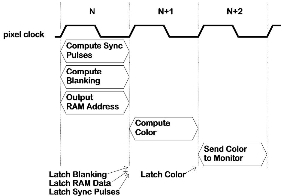
**Figure 11:** Pipelining of VGA signal generation tasks.
