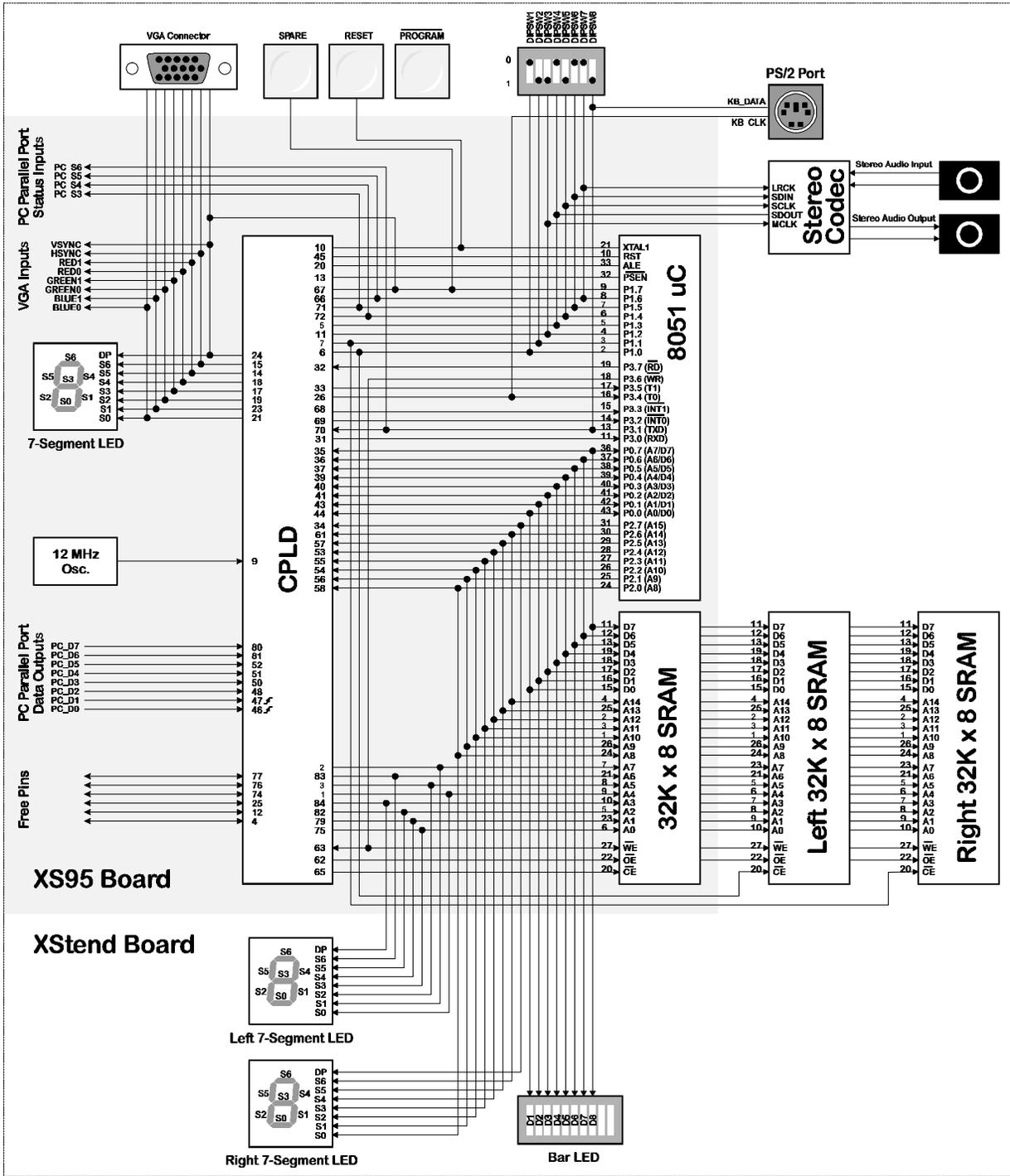
Figure 8: Programmer's model of the XS95/XStend Board combination.
